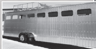
Interlocking Aluminum-Tube Walls
