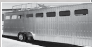
Interlocking Aluminum-Tube Walls
